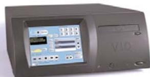
RecordIAB Console is an 8-channel rack-mountable recording console with over 10,000 channel-hours of built-in internal storage. With an 8-channel recording card, redundant hard drives, built-in CD/DVD burner and integrated touchscreen, the RecordIAB Console is an all-in-one solution for users who want the total package.
